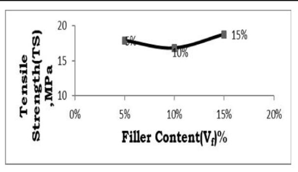
bamboo fiber reinforcement is maintained 45% and alumina is added as filler with different proportions. It can be seen that the tensile properties have become distinctly improved with the incorporation of alumina particles (15 wt %) in the matrix. The increase in tensile strength is due to the cross linking network formation between the fibers and the filler filled polymer matrix.
