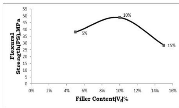
composites are probably caused by an incompatibility of the alumina particles and the polyester matrix with bamboo fiber, leading to poor interfacial bonding. However, it also depends on other factors such as the size and shape of the filler taken in the composites.
