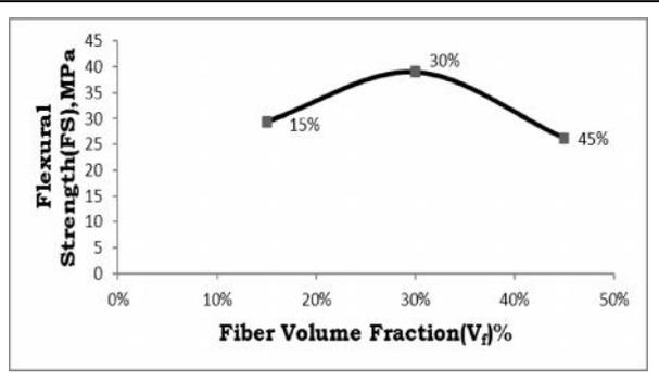
arrest points correspond to breakage and pullout of individual fibers from the resin matrix. For a composite to be used as the structural application it must possess higher flexural strength.
