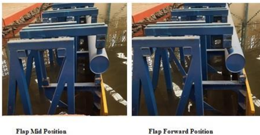
Figure 5 Suspended pendulum type wave board at CWPRS
