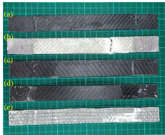
Figure 4. Failed tensile specimens after undergone test: (a) CFRP, (b) GFRP, (c) CAFRP, (d) CFRP/SRPP and (e) GFRP/SRPP
