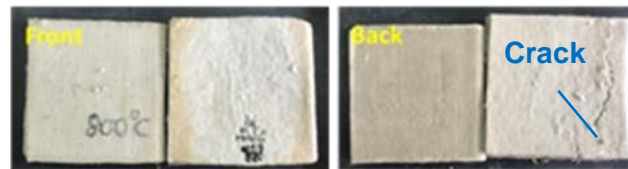
Figure 10. Effect of heat treatment for silica-fiber mats to prevent thermal shrinkage; heat treated sample (left) and non-heat treated sample (right).
