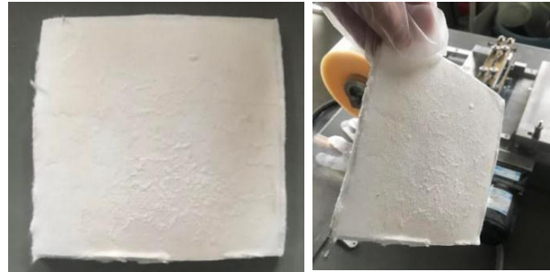
Figure 15. Appearances of composite heat insulations made by the dry process after the thermal conductivity test.
