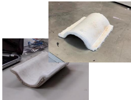
Figure 18. Trial results of press molding of composites made by the wet process (left) and the dry process (right).
