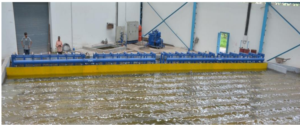
Figure.6 Generation of Regular waves in Physical model using Top hinged flap type wave generator
