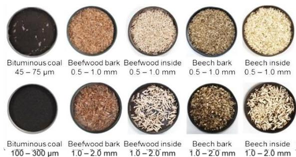
**Figure 3.** Initial samples arrange on the basket
