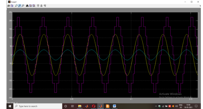
Fig. 9. Simulation results showing AC waveforms on the grid side of Solar Panel Companion Inverters (SPCI), with ideal DC voltage sources connected to the DC terminals of each H- bridge module.
